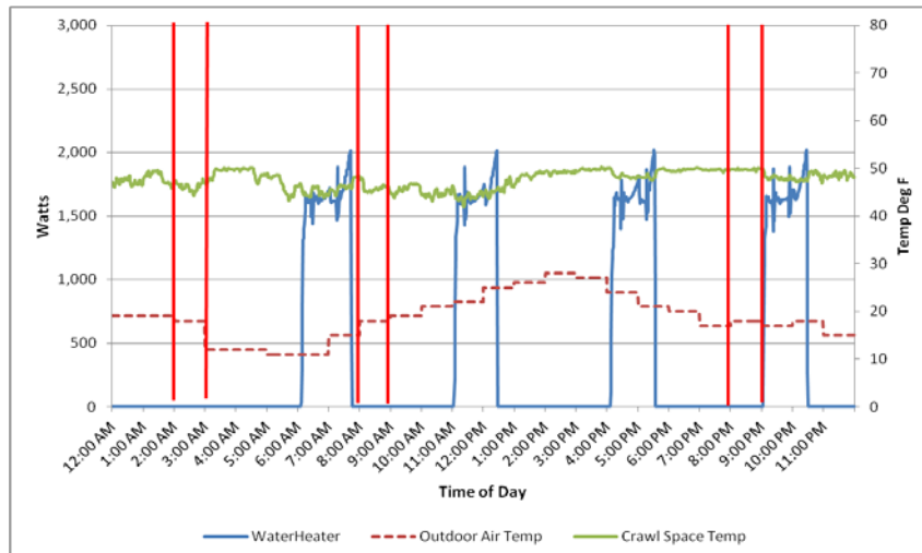
Figure 3.16. Sanden Unitary Balancing INC Power Profile: 2:00 AM, 8:00 AM, and 8:00 PM (1 hour powered-down protocol), November 16, 2014
