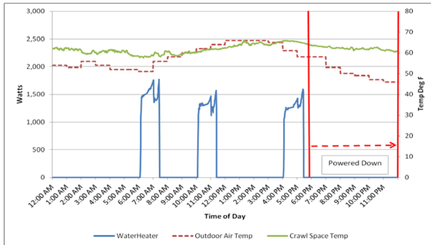
Figure 3.5. Sanden Unitary Oversupply Power Profile: First DR Event (6 hours powered-down), October 21, 2014
