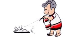
**7. SQUEEZE...** Squeeze the handle. This releases the extinguishing agent.
