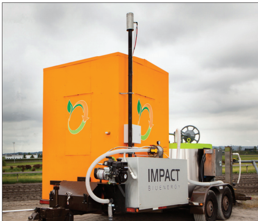
This trailered anaerobic digester is sized for a small facility with food waste. It has been named HORSE for "High-solids Organic waste Recycling System with Electrical output." Photo: Impact Bioenergy
