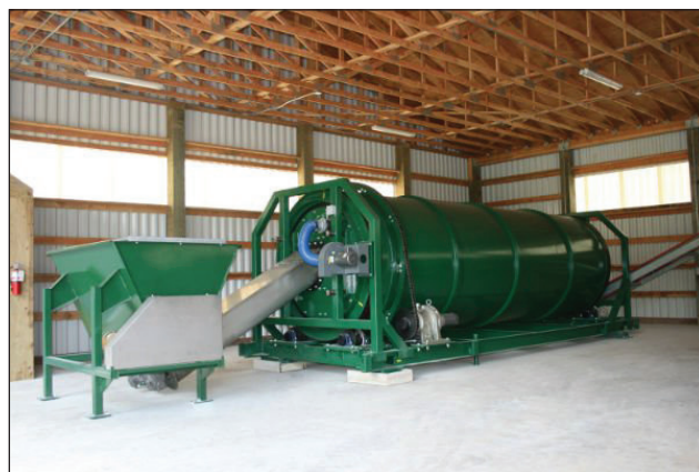
The Washington Department of Corrections has invested in composting systems at some facilities, including this drum-style rotating Envirotech composter located in Littlerock, WA. Photo: Dept. of Corrections.
