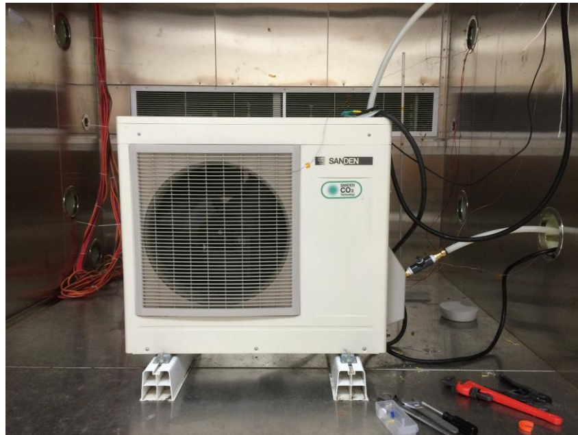
Figure 8. Sanden GAU Outdoor Unit Installed Inside Thermal Chamber
