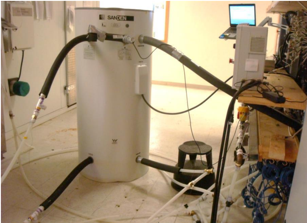
Figure 9. Hot Water Tank Instrumented and Installed Adjacent to Thermal Chamber
