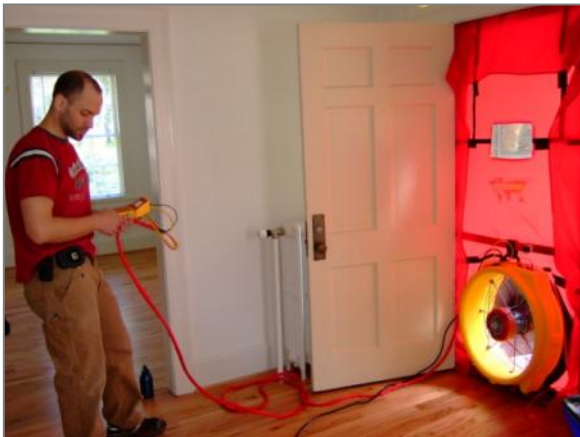
Figure 14a. Blower door testing
