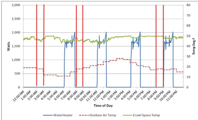
Figure 10 shows the split system performance during the 3-hour test. The operation of the heat pump is actually interrupted during this test, resulting in clear load reduction. The power use periods are longer than those of the unitary system, but they are fewer and at generally lower wattage.
