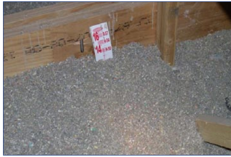
Figure 3. Researchers from Washington State University are evaluating how the bumps and vibrations of highway travel affects the settling of attic insulation installed in the factory.
