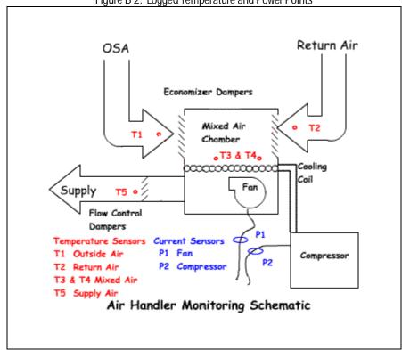
Figure B 2. Logged Temperature and Power Points
