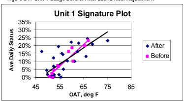
Figure B9. Unit 1 Usage Before/After Economizer Adjustment
