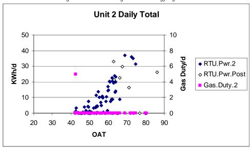
Figure B6. Pilot Building #2 RTU 2 Energy Signature
