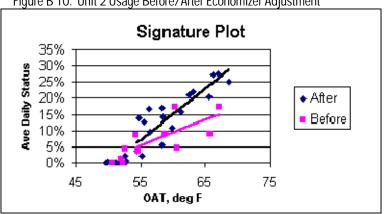
Figure B 10. Unit 2 Usage Before/After Economizer Adjustment
