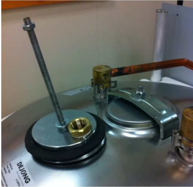
Figure 8. Custom Lid for 40 Gallon GES Tank Thermocouple Tree Access
