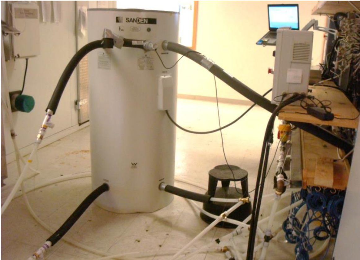
Figure 4. Hot Water Tank Instrumented and Installed Adjacent to Thermal Chamber
