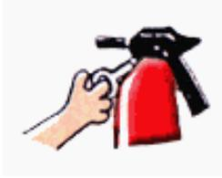
**5. PPULL...** Pull the pin. Some extinguishers require releasing a lock latch, pressing a puncture lever or other motion.
