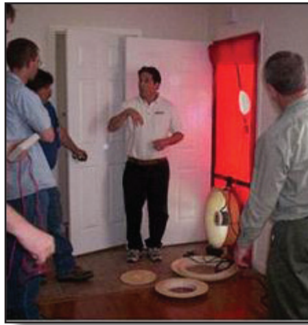
A WSU Energy Program building efficiency expert trains weatherization workers to use a blower door in a residential energy audit.
