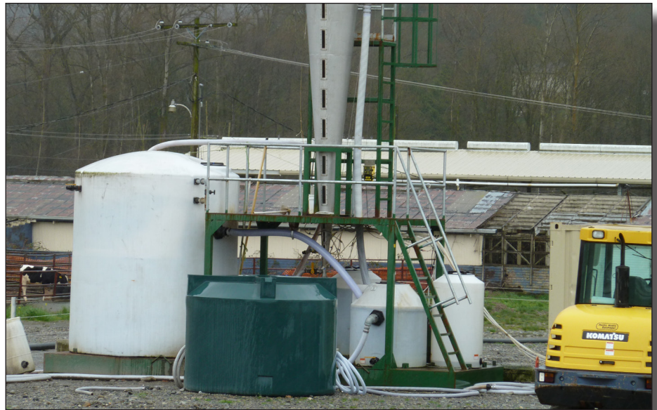
WSU tested Multifarm Harvest nutrient recovery technology at the Qualco Energy biogas facility in Snohomish County, Washington.
