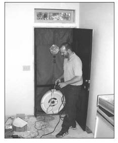
To determine the air leakage rate of a home, a blower door test is performed. A specialized fan is placed in an exterior door of the home. The fan exhausts air from the home, creating a negative pressure in the home with respect to outdoors. The target test pressure used for single point test is 50 Pascals (0.205 inches of water). The blower
